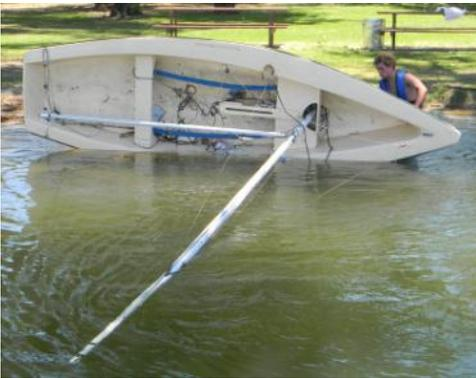
make sure they don't leak: submersion. We tested a couple of the Lake Yosemite Windmills for these photos. The rules call for two separate tanks, but the fiberglass Durabilt we tested looked as it has just one continuous tank. It is very important for floatation added to the tanks of fiberglass boats as without it they sink like a rock if there is a rupture of the tanks. Remember that ocean liner 100 years ago that was unsinkable.
